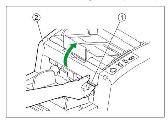
**3.** Remove dirt on the sensors with the included blower (1), then wipe the image sensor covers with the roller cleaning paper (page 48).
